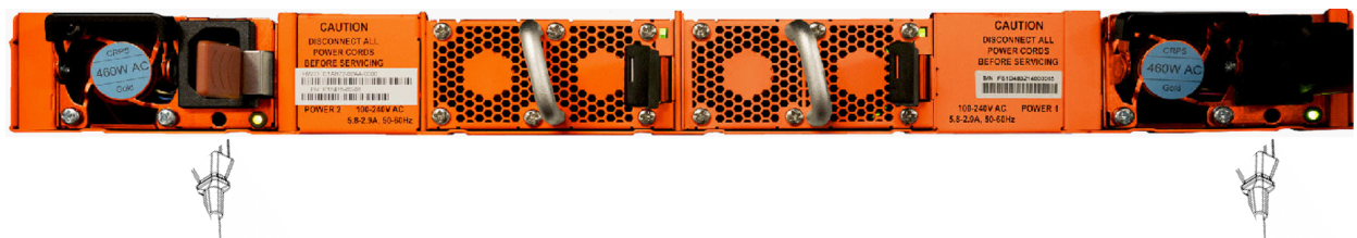
Figure 9 Connecting AC Power
